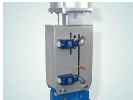
Indication of the end position OPEN / CLOSE via mechanical proximity switches with roller swivelling lever, open mounting, wiring in terminal boxes possible, optionally also for Exatmospheres.
